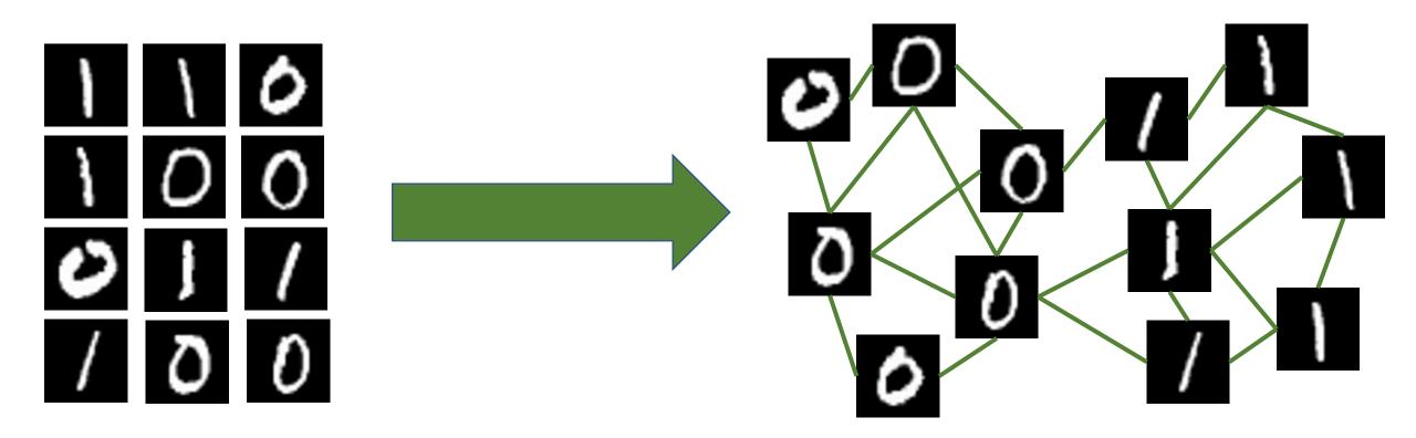
Create similarity graph according to a given distance metric [the same metric that we hope to be robust wrt]
