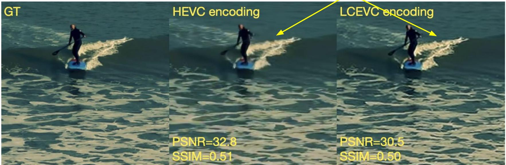
Crops from video sequences encoded using x265 and lcevc\_x265 relative to original (GT)
