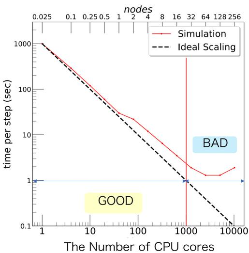
Fig.3 Strong scaling of a large galaxy simulation (Based on figure 63 in [3])
