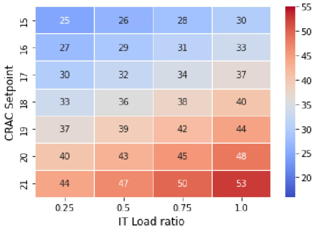
Rack Outlet Temperature(°C) as a function of IT load ratio and CRAC set point
